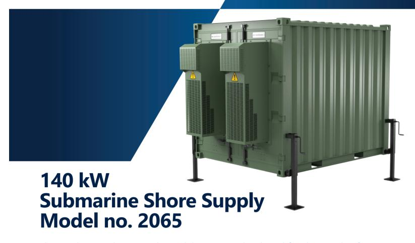
The 140 kW DC shore supply model 2065 was developed for the supply of a conventional submarine. Input supply can be either conventional 400V, 3ph, 50 Hz when using a land based shore grid, or 440 V, 3 ph, 60 Hz (in accordance with STANAG 1008 Ed. 9) when operated from a surface vessel using the respective board supply.
